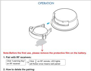
Power on the RF receiver, hold the "Learning Key" over 3 seconds until connected led lights
