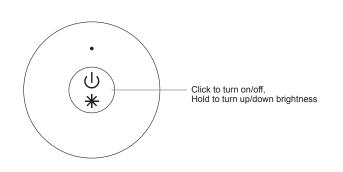
Note: This remote controls 1 zone (area) receiver, the zone can pair with countless receivers.
