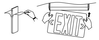
8. Insert fixture into hanger bracket and snap by spring, connect test switch, assemble LED indicator on bushing at trim plate. fix trim plate on the metal box by 2 screws.
