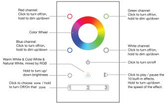
Note: This remote controls 3 zones (areas) receivers, each zone can pair with countless receivers.
