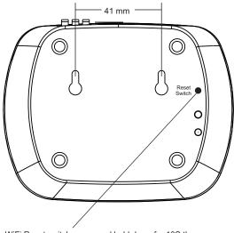
WiFi Reset switch: press and hold down for 10S then release, the blue WiFi indicator will go off and go on again, WiFi setting will be factory reset.
