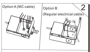
2.Open the junction box cover and remove the appropriate knockout(s) on the side panel. Insert the electrical supply cable through the knockout and secure with a cable connector (sold separately). Using quick-connect push-in terminals, connect the ground wire to the green wire terminal; black wire to black wire terminal; white wire to white wire terminal.
