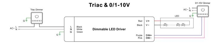
Using two ways of dimming at the same time
