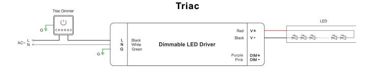
Using one dimming ---TRIAC/Phase cut dimming
