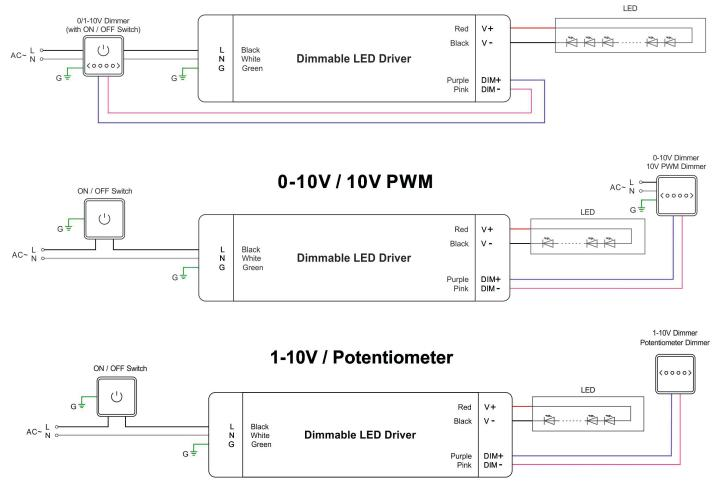
Using one dimming ---0-10/ 1-10V/ 10V PWM/ Potentiometer dimming
