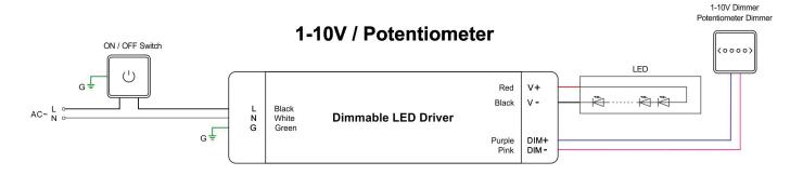
Using one dimming ---0-10/1-10V/10V PWM/ Potentiometer dimming
