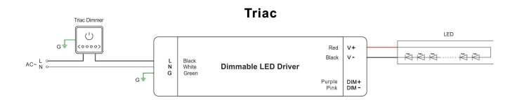
Using one dimming ---TRIAC/Phase cut dimming
